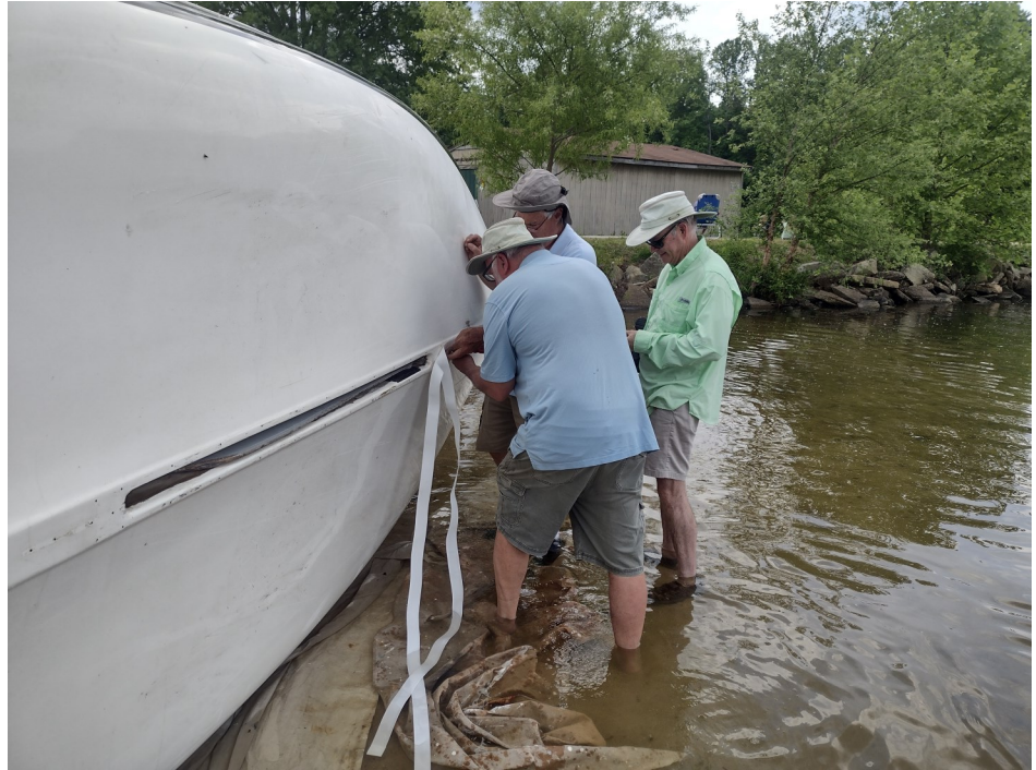
Installing the new centerboard gasket.
