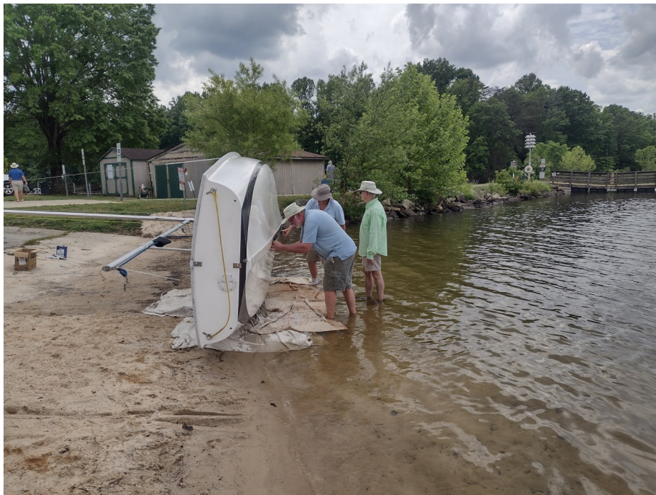
Note the cloths, laid down to protect the hull from damage by sand and to catch any dropped screws.
