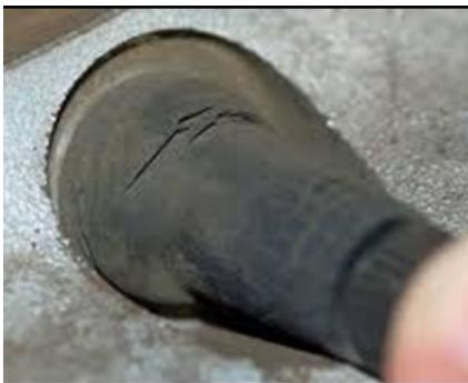
*A quick look will not tell you if your valves have cracks that have not yet caused a leak.*
