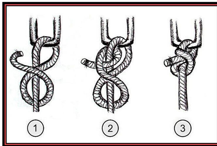
What sailing knot could you use to tie off a main or headsail halyard, hoist yourself safe and sound aloft, tie off the foot of a reefed sail or hang fenders, hammocks, or bags so that they stay in place? Not many marine knots are as compact and trustworthy as this one.
