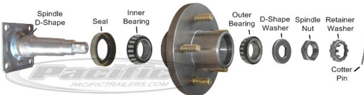
The details will vary, but the main "ingredients" are the bearings and the seal. The spindle is fastened to the end of the axle, and the wheels and tires are mounted to the long bolts in the hub, just like they are on a car. It might appear from the picture that the spindle nut and washer would keep the wheel on even if the bearings disintegrate, but they are often destroyed by heat as well.
