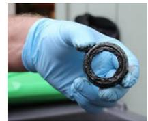
PS – how can I tell if my bearings are OK? 1. Hitch the trailer to the tow vehicle or block the wheels. 2. Jack up one wheel until the tire clears the ground. 3. Grab the wheel at 9 and 3 and rock it (don't turn it) strongly. It should not have any play. 4. Rotate the wheel and listen closely for any sound. A faint whir is OK, but any rumble, grinding or other noise is not. 5. Remove the dust caps and check for plenty of clean grease and no water.
